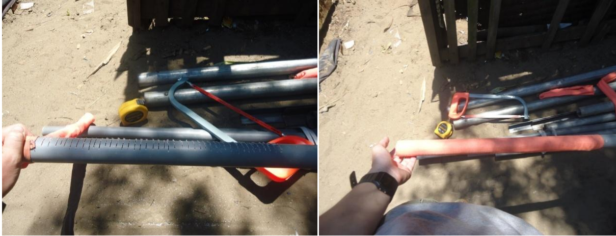
Figure 12: Base of a monitoring well. (a) Slots were cut into the base of the monitoring well to allow water to enter (picture taken by the author) (b) A polyester cloth was used as a filter (picture taken by the author)
